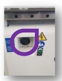
Finally shut the air valve by pulling the plunger up. If you have been using the extraction switch it off at the control panel but leave the wall isolation for air and power in the on position.
