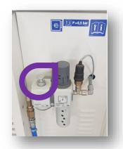
Identify machine isolator and switch on by rotating clockwise
